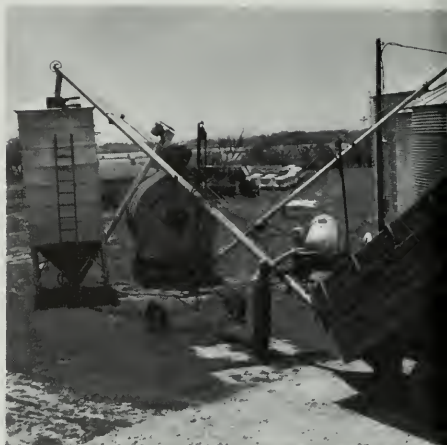
Field-harvested shelled corn must be dried before it is stored. This automatic grain drier operates 24 hours a day during the corn harvest. Wet corn is quickly transferred from the truck to a holding bin. As the automatic drier completes its drying cycle, it is loaded with wet corn from the holding bin to repeat the cycle. The dried grain is put into one of the large storage bins.
